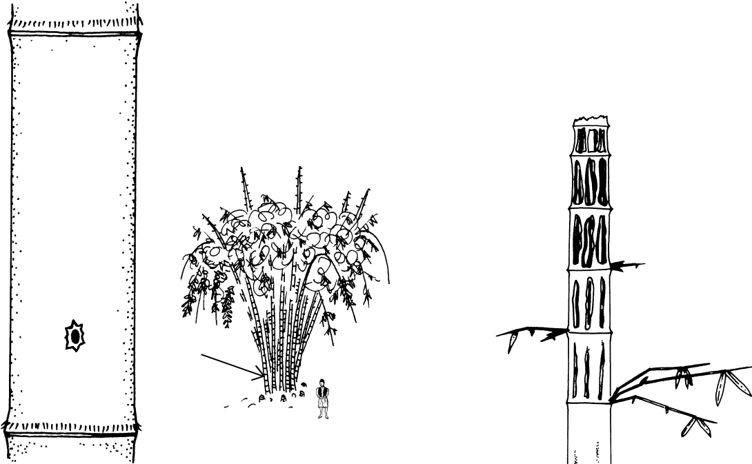
Fig (i). Location and appearance of typical entry hole.
